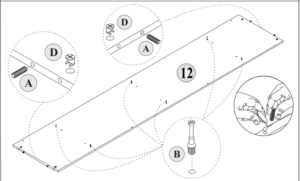
**PASSO 16: PRÉ MONTAGEM RODAPÉS (15 E 16) E TRAVESSA ROD. (17);**
