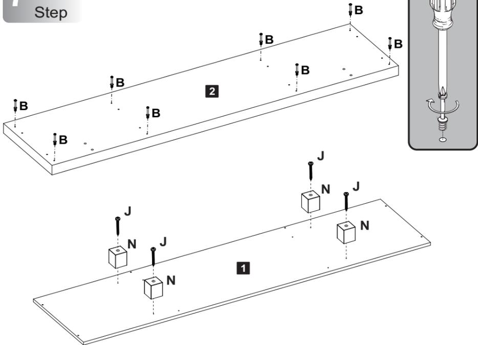
B MiniFix Ø7x30mm 08 J Parafuso Ø4,0x30mm CP 04 N Sapata Square 04
