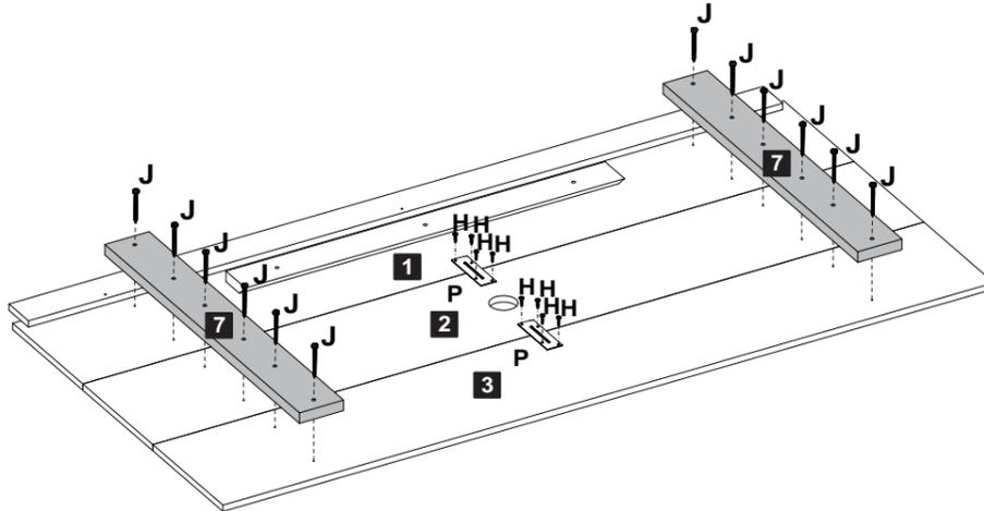
J Parafuso Ø4x30mm CP 12 H Parafuso Ø4,0x14mm CP 08 P Junção 02
